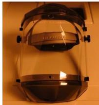
**Chemical Aprons and Face Shields Function:** For Personal protection against Chemical spills. The items are chemical resistant, NOT chemical proof. **Use:** Always wear when working with chemicals. **Location:** By the wet etch benches in the wet etch bay and in the lithography bay.
