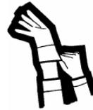
F. Put on Cleanroom Gloves. Carefully put on the first glove, touching the outside of this glove as little as possible. Put on the second glove using the previously gloved hand, taking care not to touch your skin with the gloved hand. Pull the cuff of the gloves over the sleeve of the jumpsuit so that any particles falling from your sleeves are trapped in the glove. Gloves should be worn at all times, no bare hands or fingers.
