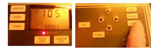
4. The display will toggle between set temp and actual temp during the heating process. Wait until it reaches the set temperature.
