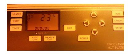
2. Press HEATER to set the desired temperature. Use the arrow keys to change the temp.
