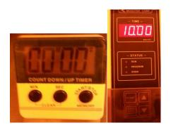
6. once baking is done, press HEATER OFF. The display should NOT toggle the set temp and actual temp.
