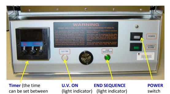
If the timer is set to a non-zero value, the ozone cleaning starts as soon as the POWER button is pressed. The "U.V. ON" light indicator is lit. The "END SEQUENCE" indicator is lit after the cleaning is finished. If the door is opened, the timer is reset, and another cleaning starts as soon as you close the door.
